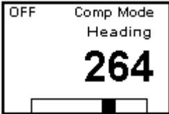
After initial power-up the Pilot displays **Comp Mode** and shows the Pilot status as **OFF**.
